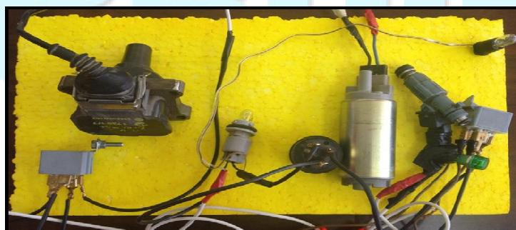
Fig. 14 b Connections of Fuel Pump Control Relay – Ignition and Injection Control relay – Flasher – Ignition Coil – Injector – Fuel pump
